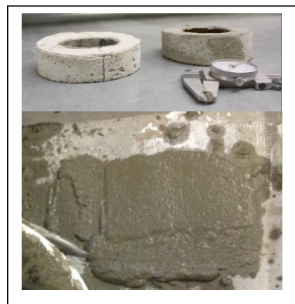
Figure 6: Top: Restrained Shrinkage Ring Test – Night Fury mix design (left), Spirit mix design (right). Bottom: Sample
